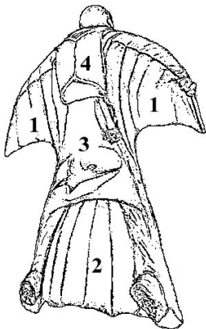
Figure 1. The Vampire 3 wingsuit in full flight. The numbered components are the (1) arm-wings, (2) leg-wing, (3) deflector, and (4) parachute.
