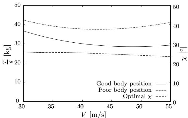
Figure 6. Minimum thrust required for level flight, and optimal  $\chi$  for level flight in the good body position.
