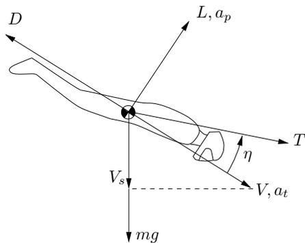
**Figure 2.** Force, acceleration, and velocity vectors of longitudinal wingsuit flight.
