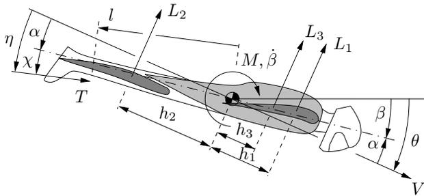
Figure 7. Cross section of the Vampire 3 wingsuit.
